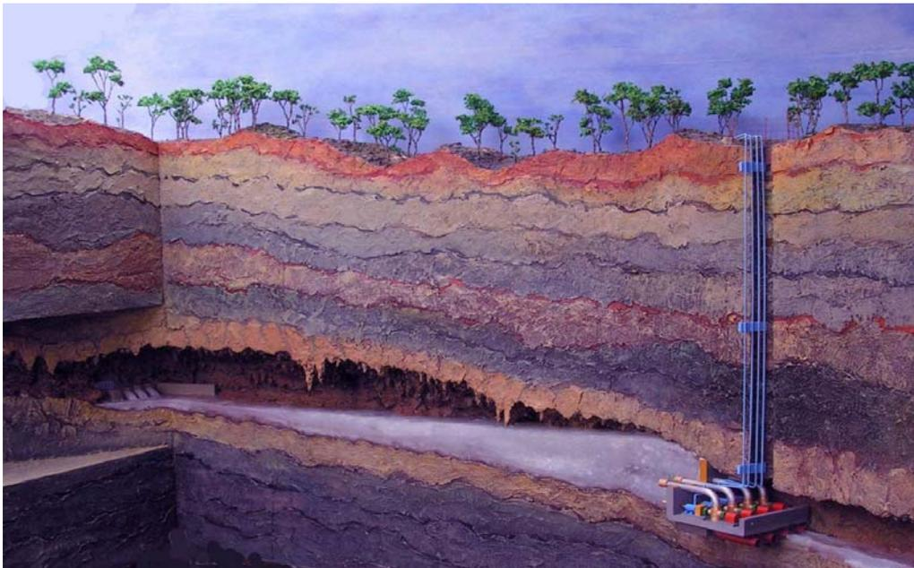
Basic sketch of the underground hydropower plant: The power station is located 100 m below the surface.
